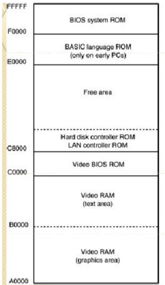
**Figure 1.4**The system area of a typical personal computer.
