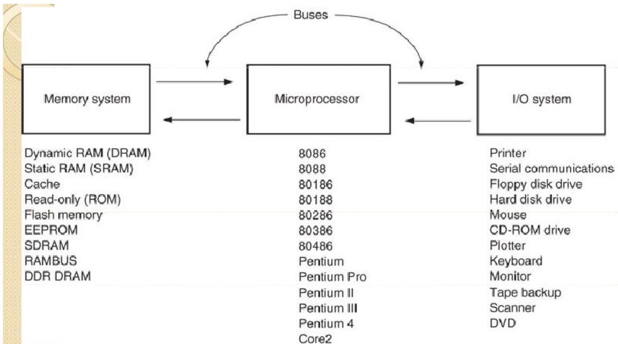
**Figure 1.1** block diagram of a microprocessor--based computer system.
